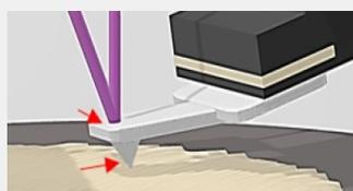
Figure 1. The tip scans the sample surface, and the SLD is used to detect the displacement of the cantilever caused by the change in surface height.
