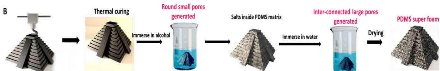
Silicon sample image 1 (above). Silicon sample image 2 (below). In this case we use a silicon material, this silicon materials were 3D printed as different objects as shown here with a formulation that shows the amount of PDS and Silicon oil added. The reason is that by varying the amount of silicon oil and salt, we are able to change the porosity.
