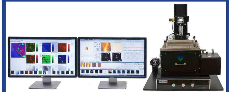
Molecular Vista develops and sells a specialized AFM instrument called VistaScope with Infrared Photo induced Force Microscopy (IR PiFM), which provides nanoscale imaging & spectroscopy.
